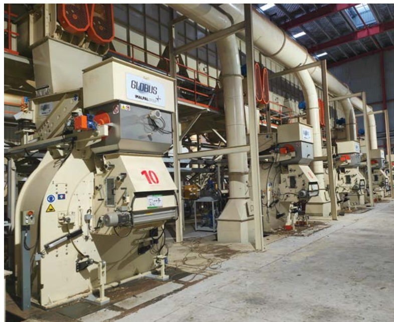
The biggest PB flaker plant in the world with 3300 m 3 /d of flakes
